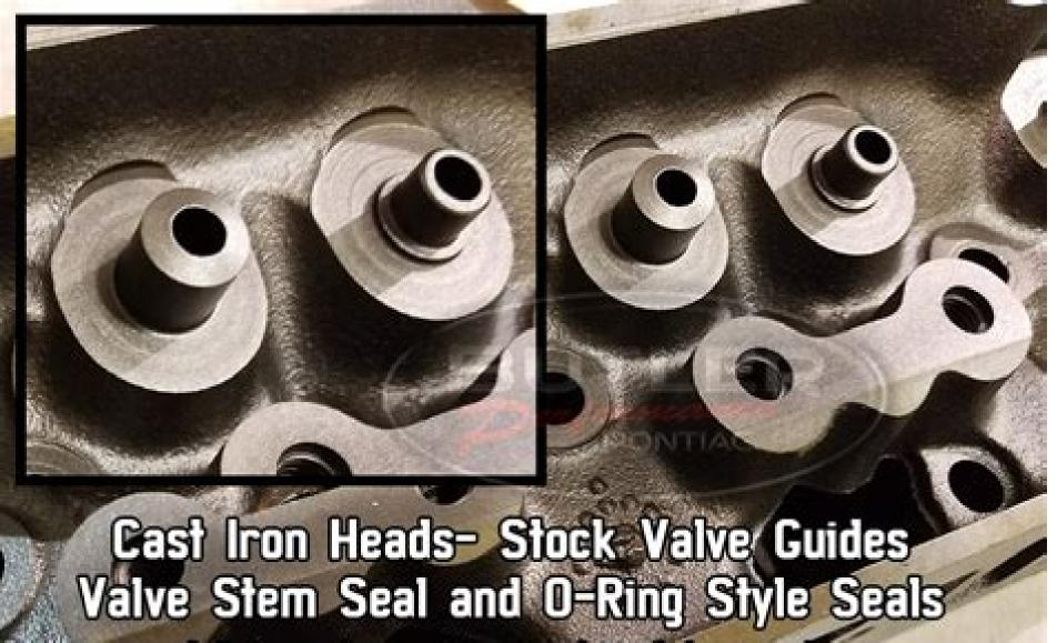
Intake valve guide machined for seals Exhaust valve guide not machined- requires o-rings
