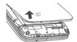
Removing or installing the back cover.
