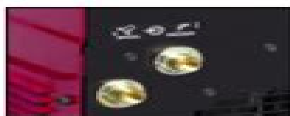
Additional Gas Solenoid – connect 2-piece TIG torch or control gas flow to a spool gun.
