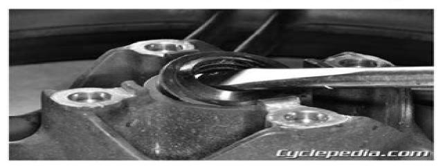
Remove the dust seals with a flat blade screwdriver. Use caution not to damage the hub.
