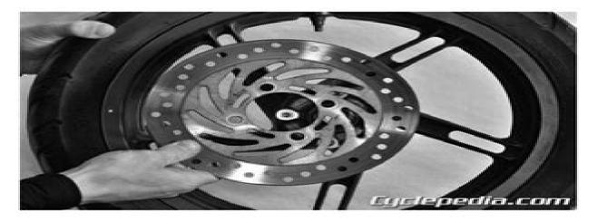
Remove the front brake rotor. See the Front Brake Rotor topic for more information.
