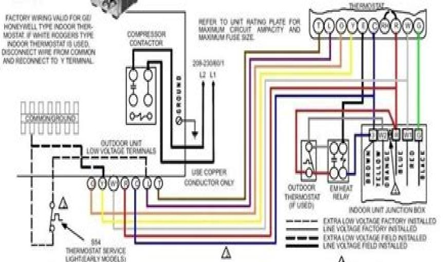
ON LATE MODEL UNITS THERMOSTAT SERVICE LIGHT CONNECTIONS ARE MADE ON DEFROST BOARD
