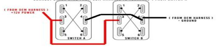
STEP 3: CONNECT TERMINAL 5 FROM SWITCH A TO RED/BLUE STRIPE WIRE CONNECT TERMINAL 6 FROM SWITCH A TO GREEN/BLUE STRIPE WIRE CONNECT TERMINAL 5 FROM SWITCH B TO RED/WHITE STRIPE WIRE CONNECT TERMINAL 6 FROM SWITCH B TO GREEN/WHITE STRIPE WIRE
