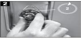
Rotate the dial to the right two tick marks. (Do not turn the dial more than two tick marks)
