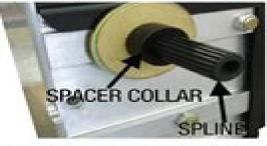
4. Install the Spline and the Spacer Collar. 5. Install the Motor onto the Spline. Install the Black Bolt and Washer onto the Motor and Tighten to Approximately 70 Foot Pounds
