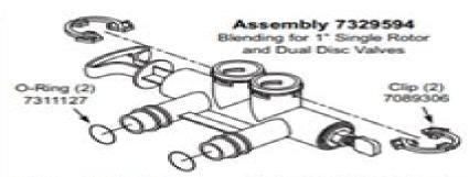
Parts: 7328530 Stem 7173016 O-Ring, Stem (4) 7175238 C-Ring 7307518 Blend Screw 7129635 Lock Nut 7329609 Clip, Blend Screw 7183590 O-Ring, Blend Screw (2)
