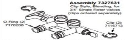
Parts: 7307534 Stem 7105013 O-Ring, Stem (4) 0502206 Retainer Ring 7129635 Lock Nut 7307518 Blend Screw 7183590 O-Ring, Blend Screw (2)
