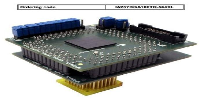
Target CPU package: QFP100
