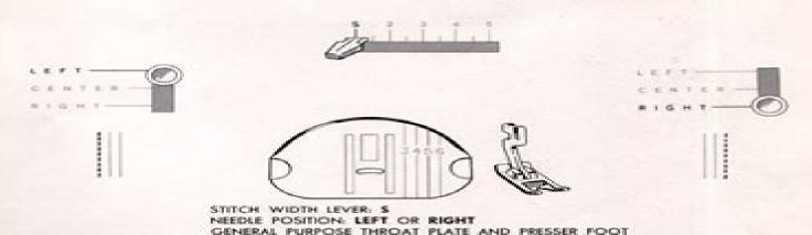
To meet special requirements, a line of stitching may be placed to the left or right of center. LEFT needle position setting locates stitching at the extreme left; RIGHT needle position setting locates it at the extreme right.
