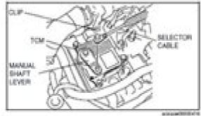
3. Remove the selector cable from the cable benchet.
