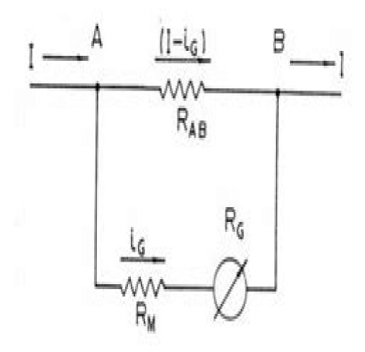
Figure 3: a galvanometer as a voltmeter
