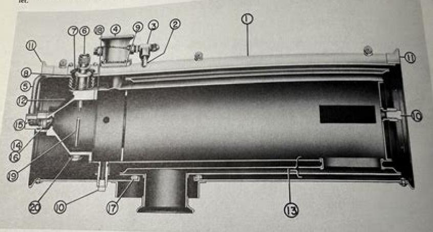
Figure 2 — Cutaway View of 20C61 Heater
