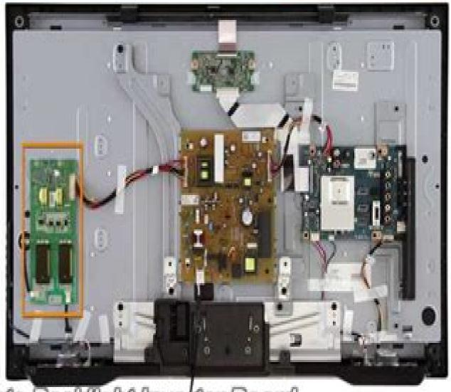
Locate Backlight Inverter Board
