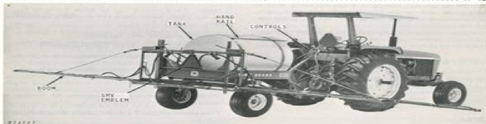
John Deere 535 Sprayer with 30-Foot (9.2 m) Boom
