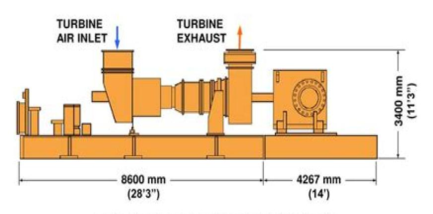
Typical Package Weight = 52 255 kg (115,200 lb) Width = 2700 mm (9')
