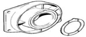
73. MD17: Smear both thrust washers with grease and place one of them on the inner side of the bearing shield, turning the flat side towards the main bearing. Ensure that the lug on the washer fits into the recess in the shield. Fit the bearing shield onto the engine and tighten the screws.
