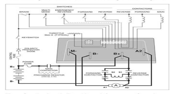
The configuration shown in Figure 3 is a typical arrangement for a series motor. Curtis controllers are designed for use in a wide range of applications, and accordingly can be installed in a variety of ways to best meet customer needs.
