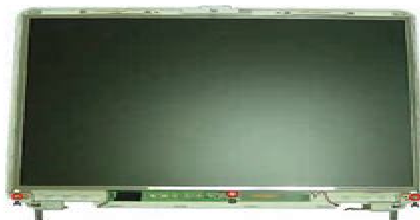
Fig. 29 Removing the LCD panel screws
