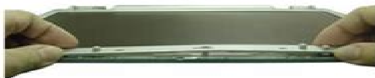
Fig. 28 Removing the LCD front cover
