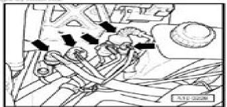
Detach coolant hose (top) from radiator by releasing retaining clip -arrow-.
