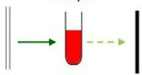
2. Light passes through a slit to form a narrow beam
