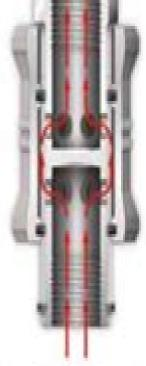
In the On position, the air coming from the air source passes through the holes on the stem of the valve.
