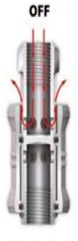
In the DFF position, the air in the circuit passes through the holes on the stem and automatically exits to the atmosphere.
