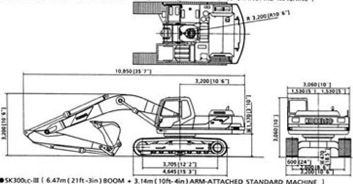
◆SK300Lc-III ( 6.47m ( 21ft -3in ) BOOM + 3.14m ( 10ft-4in ) ARM-ATTACHED STANDARD MACHINE ]
