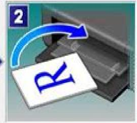
Keeping the printed side facing up, rotate the paper 180 degrees so that the front edge of the printed paper faces away from you.
