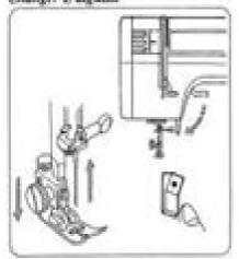
Raise the needle by turning the balance wheel toward you and lower the preser foot.
