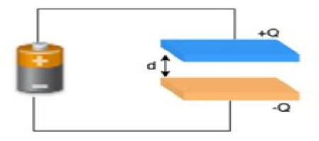
The ratio of the magnitude of charge that builds up either plate and the potential difference that is applied to the plates gives a term called the capacitance C of the capacitor. The SI units of capacitance are Farads. F.
