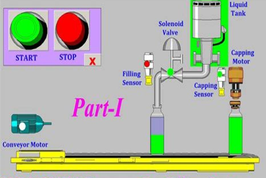
PLC & SCADA Program For Filling System
