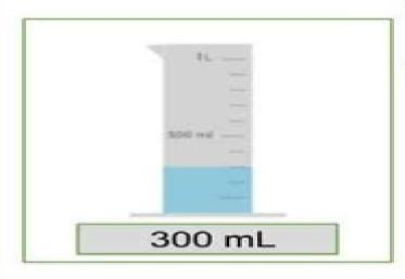
Read the volume of the liquid by getting the measurement of the upper portion of the liquid
