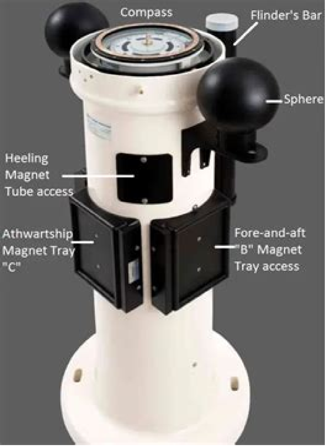
Fig 13: Magnetic Compass Binnacle with Correctors
