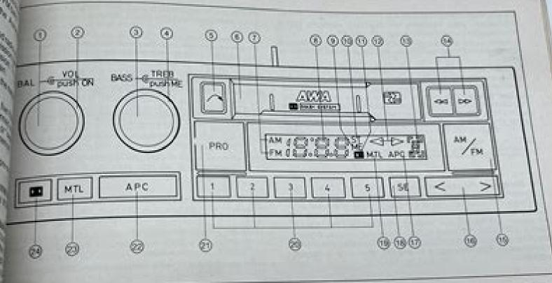
Metal tape equalizer button: When playing CrOz, or metal ction will only open as press button for tape equalization (70µs). normal tapes (120µs) press button again.
