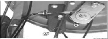
. With ground speed control lever in fast position, the drive belt (A) is taut and idler spring (8) on end of ground speed control cable is extended approximately 25mm (1 in.).
