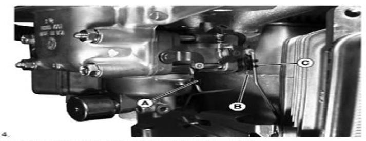
Rotate clip (A). Disconnect choke rod from choke shaft.
