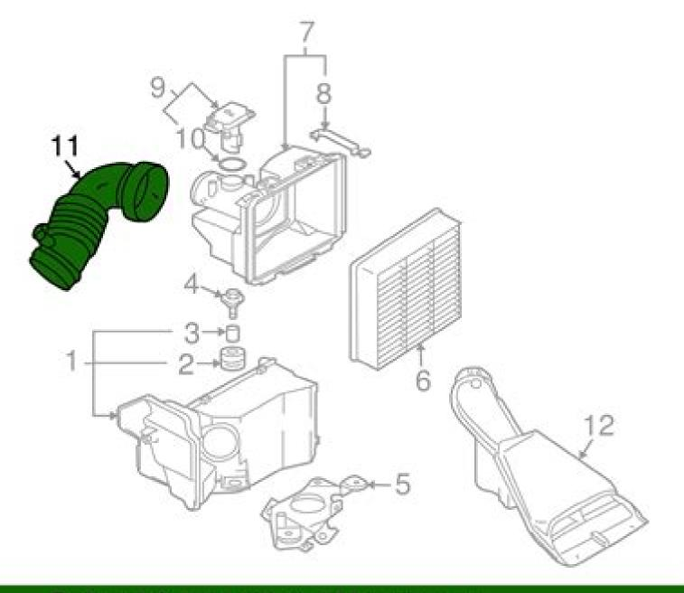
Part or sub-assembly is #11 in diagram Diagram may not be specific to your vehicle
