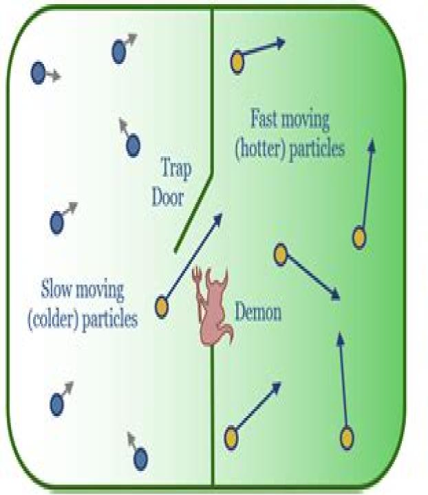
Maxwell's Demon opens and closes the trap door partitioning two chambers, in order to move all of the 'hot' particles to the right-hand side and all of the 'cold' particles to the other side, using "nothing but information".
