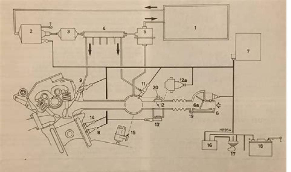
Fig. 3.29 L-Jetronic fuel injection system (Sec 22)
