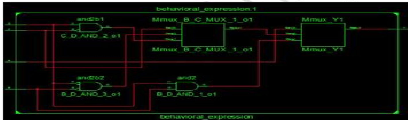
Figure 3.4 RTL Schematic of the given expression using behavioural modelling
