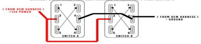
STEP 3: CONNECT TERMINAL 5 FROM SWITCH A TO RED/BLUE STRIPE WIRE CONNECT TERMINAL 6 FROM SWITCH A TO GREEN/BLUE STRIPE WIRE CONNECT TERMINAL 5 FROM SWITCH B TO RED/WHITE STRIPE WIRE CONNECT TERMINAL 6 FROM SWITCH B TO GREEN/WHITE STRIPE WIRE
