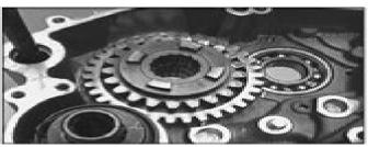
Take the 3rd gear/sliding gear and the 1st gear/idler gear out of the engine housing together with the needle bearing and the stop disc.
