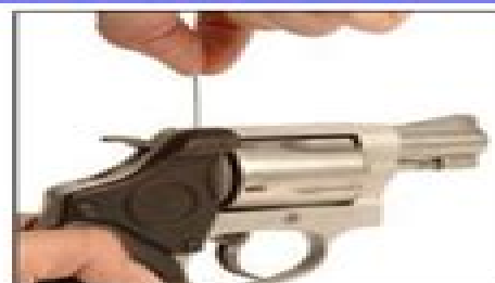
The hole at the top adjusts elevation (vertical alignment).*
