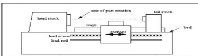
head stock - this end of the lathe contains the driving motor and gears. Power to rotate the part is delivered from here. This typically has levers that let the speeds and feeds be set ways - these are hardened rails that the carriage rides on.
