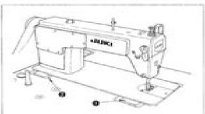
Fit hings into the opening in the machine bed, and fit the machine head to table rubber hings hefore placing the machine head on cushious on the four corners.
