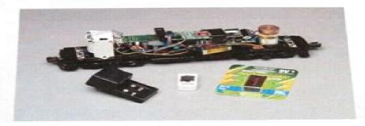
Although LtTH circuitry continuously recharges the battery whenever you run your locomotive, the original factory-installed. NiCad (nickel cadmium) battery deteriorates with age until it can no longer hold a charge or reach its full voltage capacity, no matter how long you charge it. At this point, the battery must be replaced.
