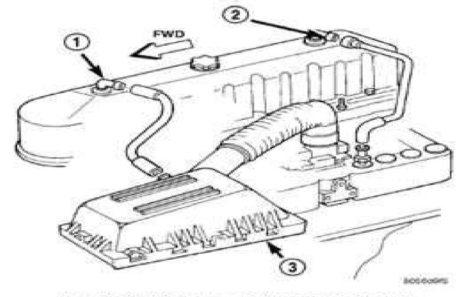
Fig. 2 CCV System-4.0L Engine-Typical
