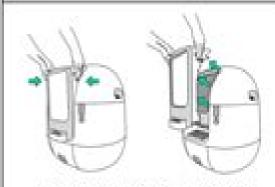
Remove the door frame by holding down the clips inward on both sides of the top of the door frame at the same time, and install the same way.
