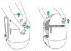
Hold the top cover with one hand, press the side class of the top cover with the other hand, after the class is loosened. Eff: the top cover upward to complete disassembly
