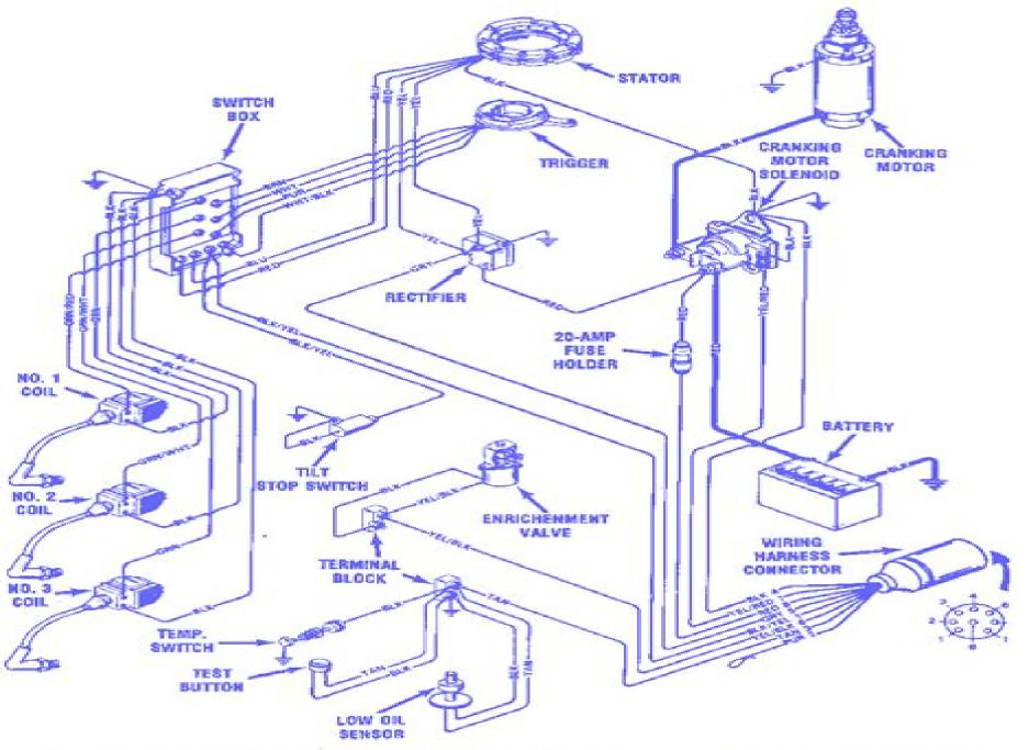
Functional wiring diagram for the 3-cylinder Model 75 and 90hp powerheads WITHOUT low oil warning module. Wire color code identification is indicated.
