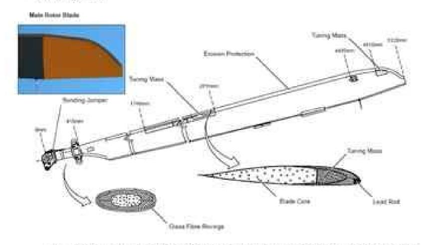
a. The four main rotor blades are manufactured from fiber-reinforced plastic and are directly connected to the rigid titanium rotor head.
