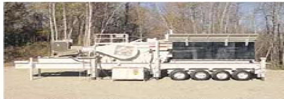
The extra-wide C3055 assembled on a portable, fully mobile crushing plant.
