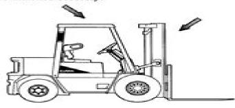
Check the overhead guard for damage. Be sure that it is properly positioned and all mounting fasteners are in place and tight.
