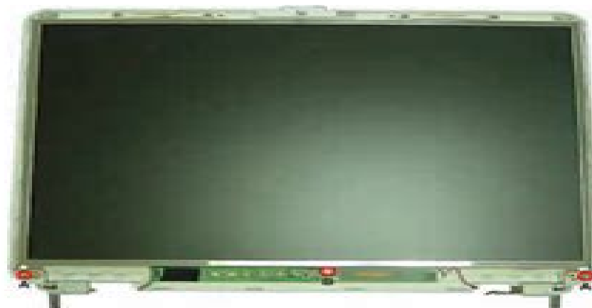
Fig. 29 Removing the LCD panel screws
